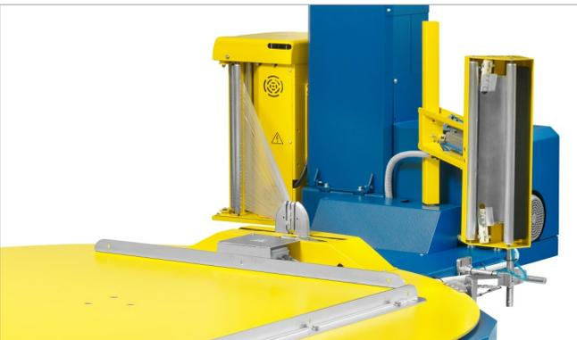
Incorporating all belonging functions of attaching, clamping, cutting and wiping the film end to the package.
